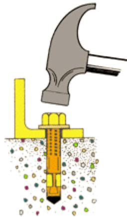
2. Place nut on the end of the wedge anchor (to protect the threads of the wedge anchor during installation) Drive wedge anchor into drilled hole through fixture so that nut is flush with fixture.
